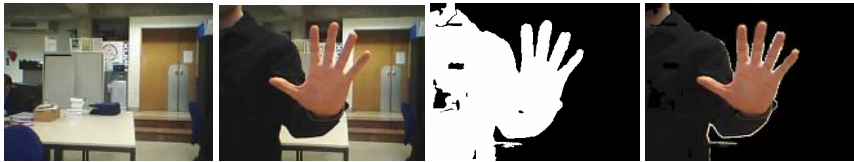
Fig. 2. Subtracting the background. From left to right: The original background; A user in the foreground; Resulting background subtraction mask; Subtracted background.
