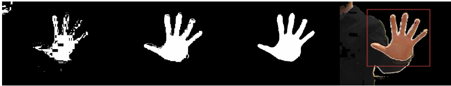
Fig. 3. Extracting the hand contour. From left to right: the CAMSHIFT algorithm histogram back projection result; Result after YCrCb re-sampling; Result after morphological smoothing; Result after contour vectorisation and mixture with the foreground image.
