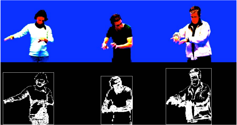
Fig. 3. Output of a patch made for comparative analysis of three separate air piano performances, showing a novice, semi-expert and expert performer from left to right. The quantity of motion images with bounding boxes, are very useful when the movements are so subtle that they are difficult to see in the original video.
