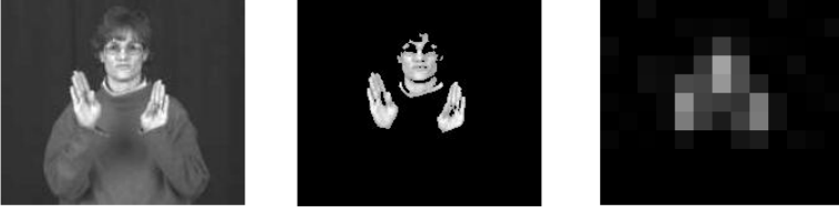
Fig. 2. Example of the features used by the classifier: original image (left), thresholded image (center), and down-scaled image (right)
