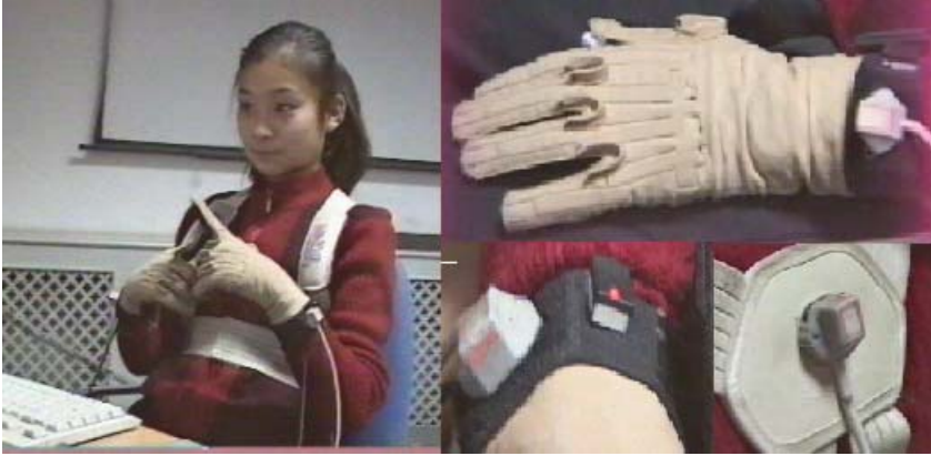
Fig. 1. The Dataglove and the 3-D tracker used in our system. Three receivers are fixed on two hands and the back respectively.
